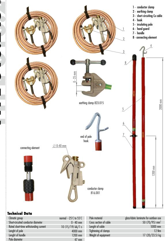
The short-circuiting (earthing) equipment is designed for short-circuit making and earthing of the circuit in networks with an earthed node of the nominal
